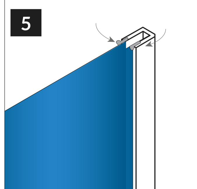
Subsequently, the glass in the U profile is secured on each side using seals. (See Fig. 5.)
