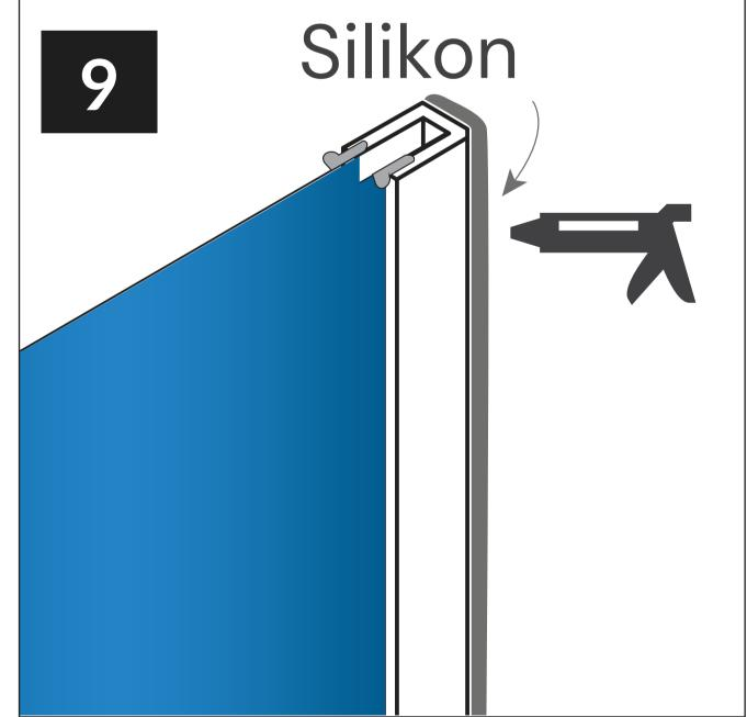
All parts are dried, degreased, and the resulting 3 mm gap between the fixed glass and the floor is filled with silicone, which is included in the delivery. Similarly, any unevenness between the U profile and the wall on the inside is sealed with silicone. (See Fig. 9 and 10.)
